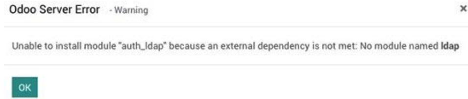
Figure 2.2 – Warning for external library dependency
